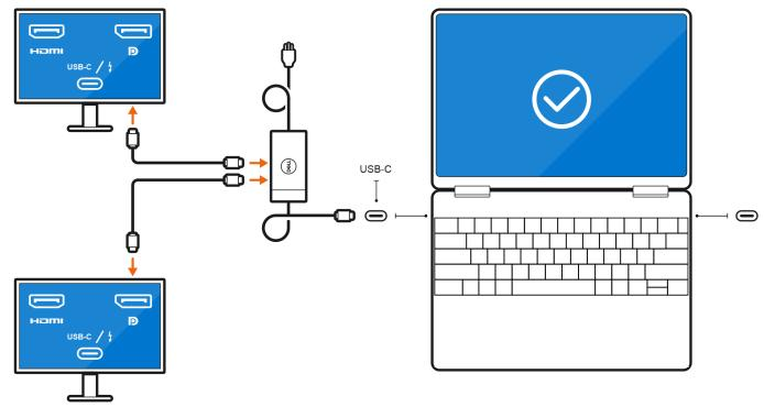
• Connect up to three external displays using a docking station.
