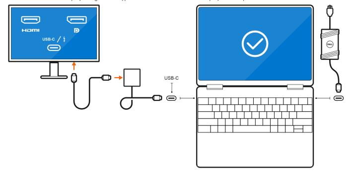
• Connect up to two external displays using a docking station.
