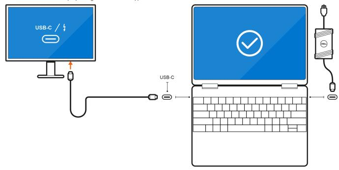
• Connect an external display using a USB Type-C to Thunderbolt/HDMI/DisplayPort adapter.
