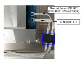
S16 Tear off 6 tapes from the backlight wires on panel (See blue mark)
