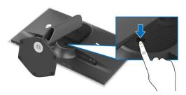
Lift the stand assembly up and away from the monitor.
