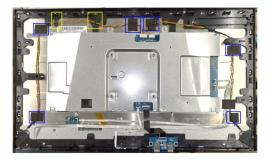
S17 Unlock 2 screws to disassemble "Main SHD" from Panel
