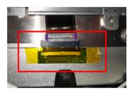
S12 Unlock 7 screws to disassemble Middle Frame and "ASSY BKT CHIN" (See blue marks)
