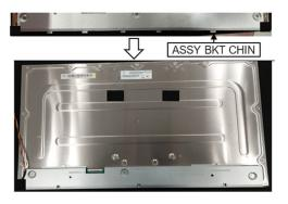
S14 Tear off an acetate tape from the connector of backlight on panel
