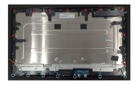
(Screw Torque-MF to Chin: 2.0±0.5 kgf) (Screw Torque-MF to panel: 2.0±0.5kgf)
