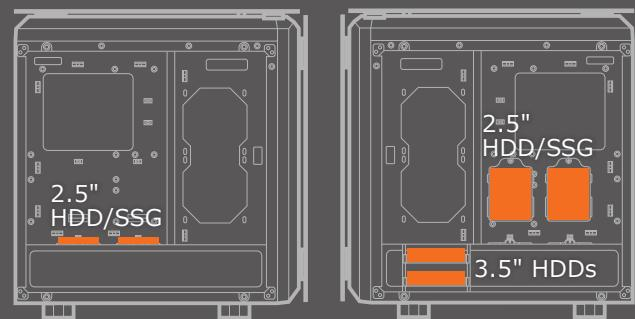
Two 3.5" HDDs and four 2.5" HDD/SSG
