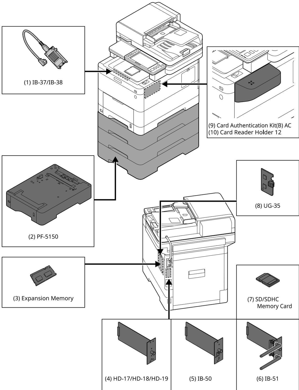
1 IB-37/IB-38 <Wireless network interface (USB: 5GHz/2.4GHz)>
