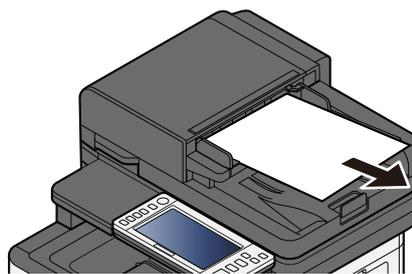
**2 Open the Document Processor cover and remove the jammed paper.**
