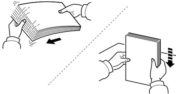
Fan the paper, then tap it on a level surface. In addition, note the following points.
