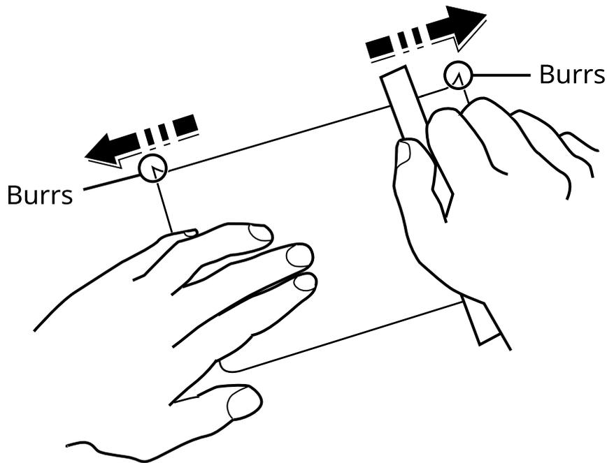
Before loading Hagaki (Cardstock) into the multipurpose tray, fan them and align the edges. If the Hagaki (Cardstock) paper is curled, straighten it before loading. Printing onto curled Hagaki (Cardstock) may cause jams.
