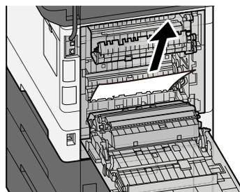
**5** Open cover A2 and remove the jammed paper
