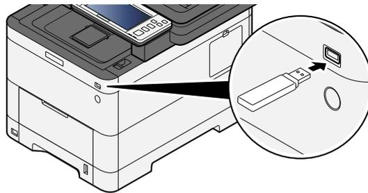
When the machine recognizes the USB drive, the message "USB Drive is recognized. Displaying files." appears.
