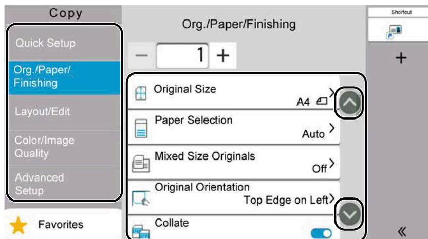
When an On/Off Flipswitch is displayed for a function, select the switch to change between ON and OFF.
