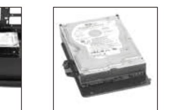
Fix the bracket with screws
