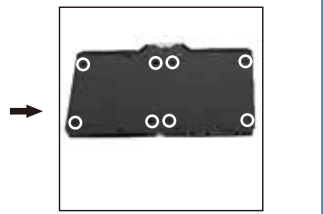
Fix them with M/B screws from the back of bracket
