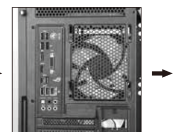
Fit I/O into I/O slot
