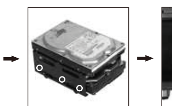
Push HDD into the bracket
