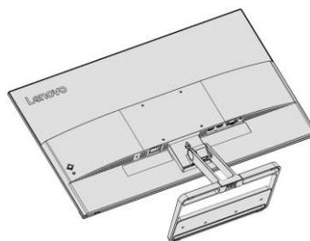
Step 3: Remove the base and stand from the display, see "Removing the Display Base and Support Arm" on pages 2-9.
