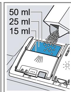
If you are using tablets, one is enough. Insert the tablets in a horizontal position.
