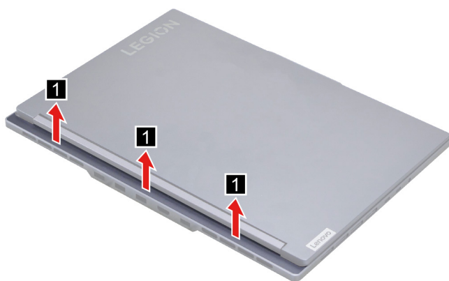
Figure 31. Remove the strip cover mylar
