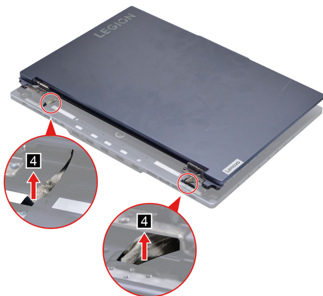
Figure 34. Take out the EDP cable and the camera cable to remove the LCD module
