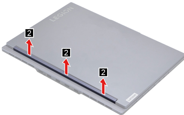
Figure 30. Remove the hinge cover with antenna
