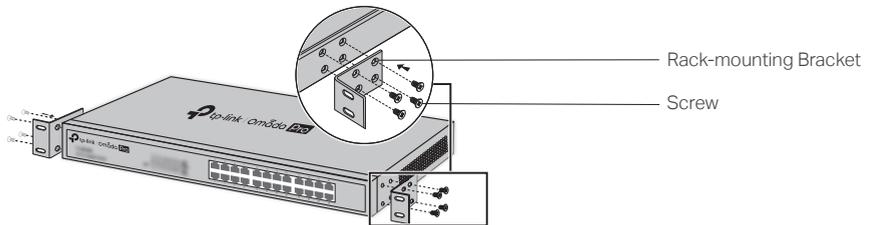
3. After the brackets are attached to the device, use suitable screws to secure the brackets to the rack, as illustrated in the following figure.
