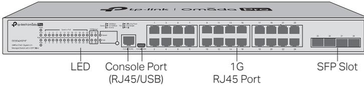
The front panel of S5500-24GP4XF is shown as the following figure.
