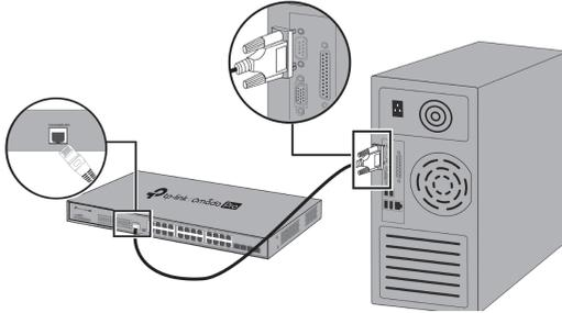
Connect the console (USB) port of the device with your computer by the USB cable (not provided) as the following figure shows.
