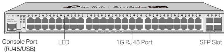
The front panel of S5500-48GP4XF is shown as the following figure.
