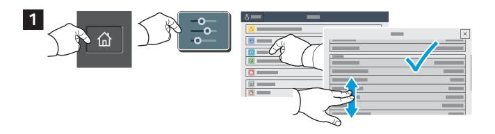
Note the printer IP address on the touch screen. If the IP Address does not appear in the top of the touch screen, press Home, touch **Device > About** then scroll to check the IP Address.
