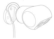
5. Slide the camera onto the mounting plate and make sure it is attached securely.
