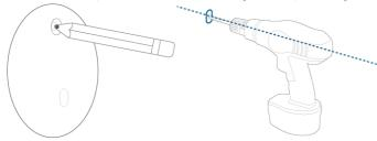
2. Hold the mounting plate on the wall and make sure the "UP" arrow is pointing up. Secure the mounting plate to the wall or ceiling with the screws.
