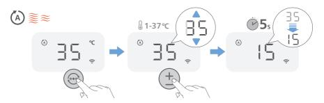
**Auto mode:** In this mode, your device will do the work for you. Based on the sensor data that measures and tracks the temperature in your room, your device automatically selects the heating speed to keep your room comfortable.
