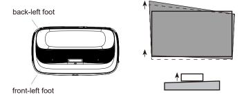
2. Now, rotate the TV clockwise so that the bottom of the image is parallel with the screen.
