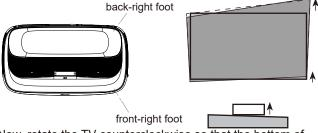
Now, rotate the TV counterclockwise so that the bottom of the image is parallel with the screen.
