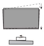
Repeat the steps above until the top of the image is parallel with the screen. 4. If the upper-right corner is inside the screen after adjusting, use the wrench to rotate the front-right foot and the back-right foot counterclockwise to the same height, and rotate the TV clockwise, to make the image parallel with the screen.
