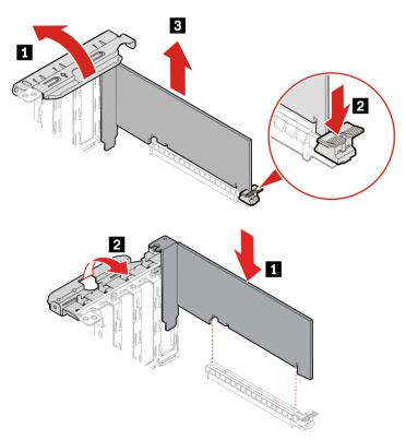
**Note:** During the installation, ensure that you align the PCI-Express card to the slot and press down until the latch is fully engaged with a click.
