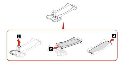
Note: When installing the M.2 solid-state drive and the heat sink, remove the film (if any) that covers the thermal pad.
