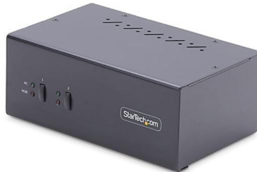
This Dual-Monitor KVM Switch enables users to switch between two desktops that are USB-A and DisplayPort enabled. It allows for sharing of dual-4K 60Hz DisplayPort monitors, a keyboard and mouse, two USB 5Gbps devices, and two USB 2.0 HID devices.
