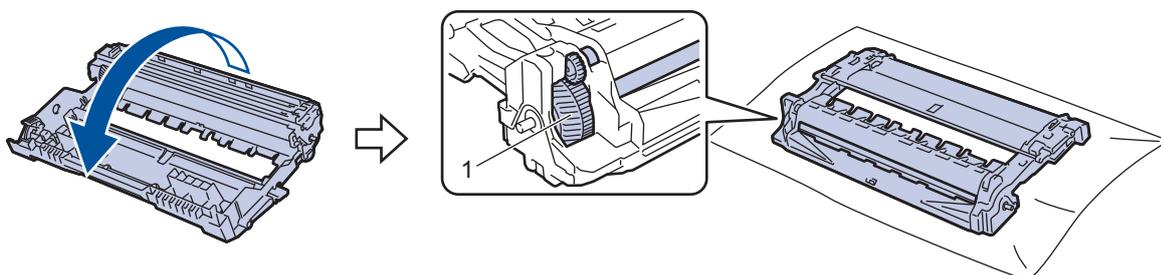
12. Use the numbered markers next to the drum roller to find the mark on the drum. For example, a dot in column 2 on the check sheet means that there is a mark in drum region "2".
