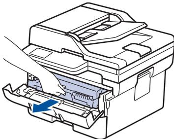
10. Push down the green lock lever and take the toner cartridge out of the drum unit.
