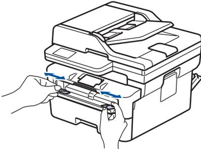
4. Using both hands, place one sheet of paper in the manual feed slot until the front edge touches the paper feed roller. When you feel the machine pull it in, let go.
