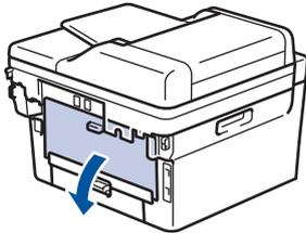
3. Pull the blue tabs at the left and right sides towards you to release the fuser cover.
