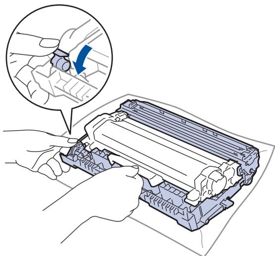
11. Turn the drum unit as shown in the illustration. Make sure that the drum unit gear (1) is on the left side.
