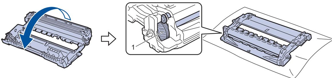
10. Use the numbered markers next to the drum roller to find the mark on the drum. For example, a dot in column 2 on the check sheet means that there is a mark in drum region “2”.
