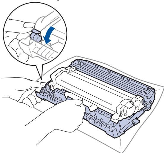
9. Turn the drum unit as shown in the illustration. Make sure that the drum unit gear (1) is on the left side.
