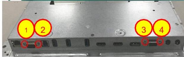
Use a Philips-head screwdriver to remove 8 screws for remove the Power board.
