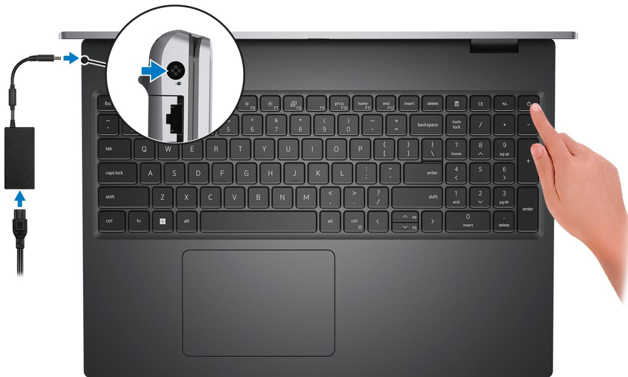
**i** **NOTE:** To conserve battery power, the battery might enter power saving mode. Connect the power adapter and press the power button to turn on the computer.
