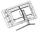
While keeping the release button pressed, tilt the stand and slide it out.
