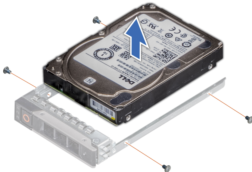
Figure 105. Removing the drive from the drive carrier
