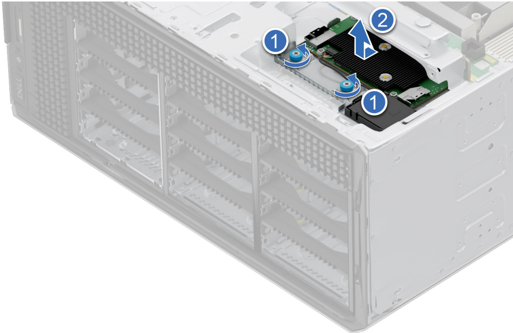
Figure 96. Removing the front PERC module from the 3.5-inch drive backplane
