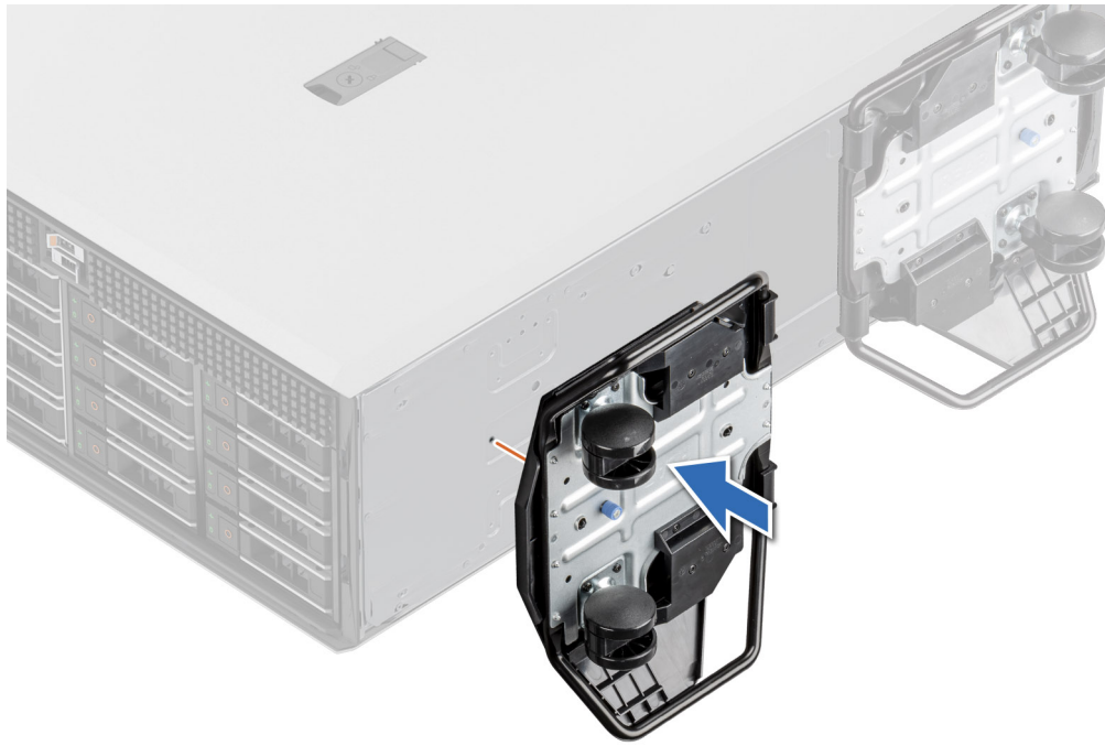
Figure 27. Installing caster wheels
