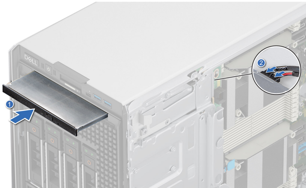
Figure 128. Installing the optical drive
