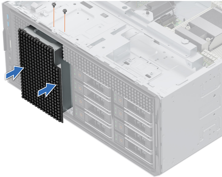
Figure 118. Installing the NVMe drive bay blank
