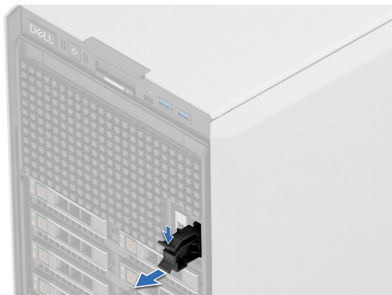
Figure 145. Removing the BOSS-N1 card carrier blank
