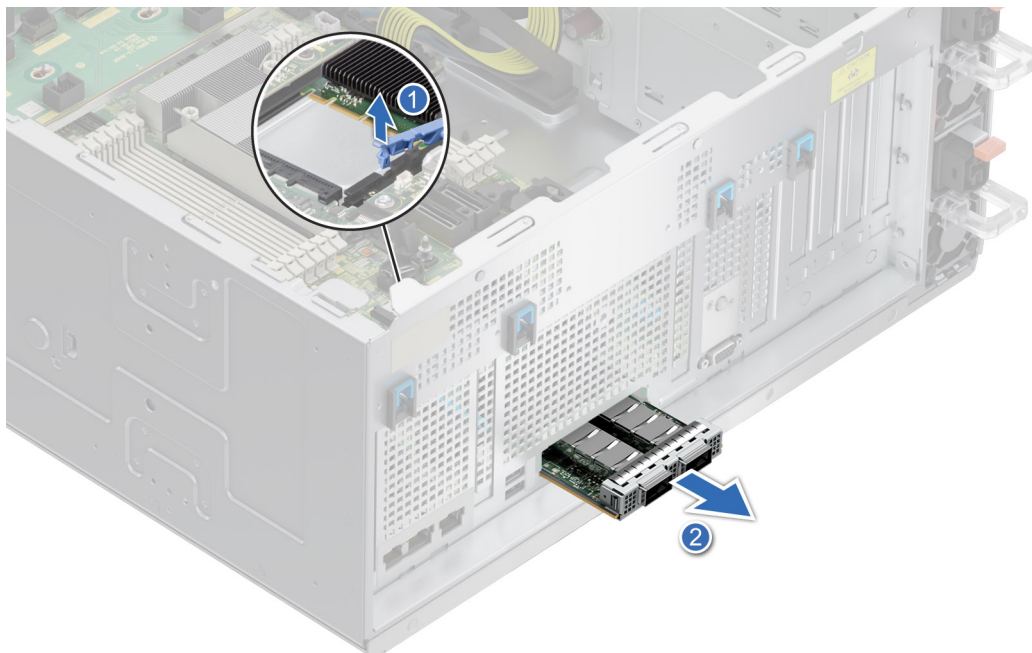
Figure 173. Removing the OCP card
