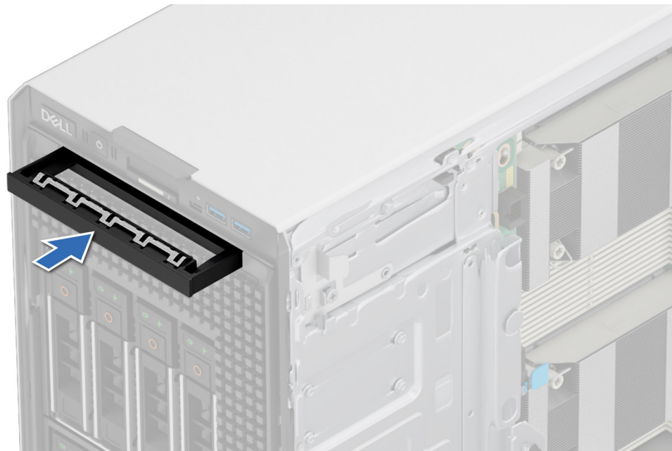
Figure 126. Installing the optical drive blank
