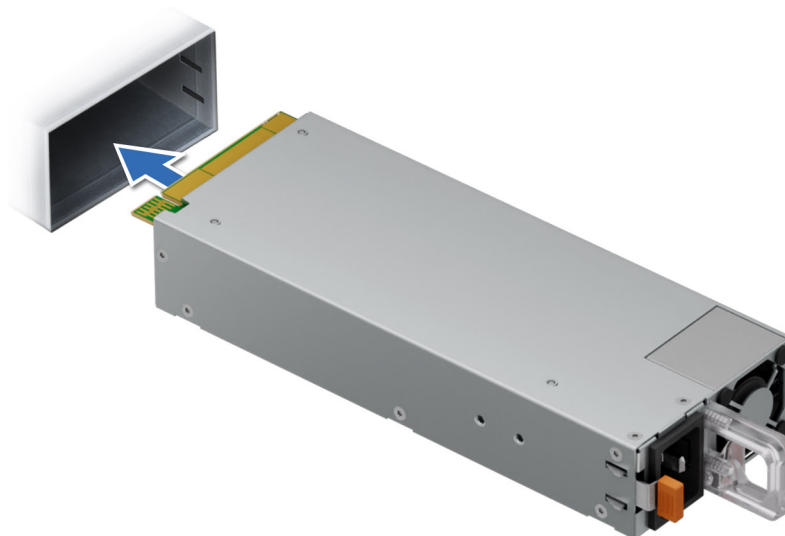
Figure 191. Installing a 86 mm power supply unit
