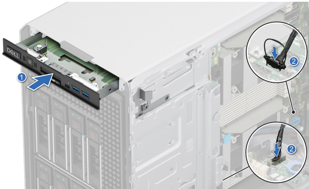
Figure 134. Installing the front IO module
