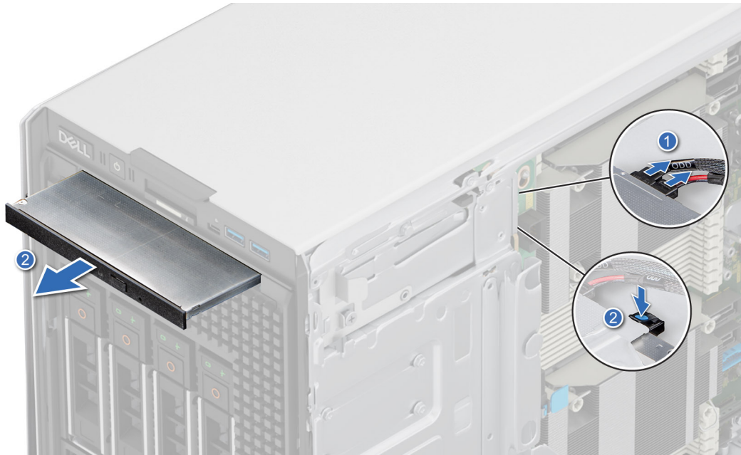
Figure 127. Removing the optical drive
