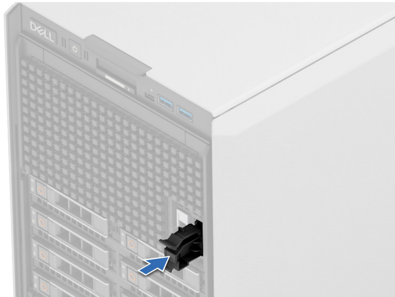
Figure 144. Installing the BOSS-N1 card carrier blank
