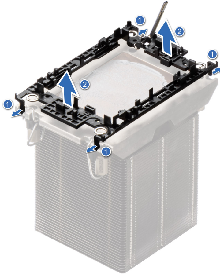
Figure 164. Removing the retaining clip
