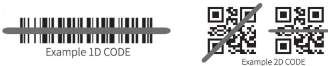
The closer to the barcode, The beam becomes smaller farther away from the barcode, The beam becomes larger. If the bar code is small, the scanner should be close to the barcode. If the barcode is larger, the scanner should be further away from the barcode, making it easier to read the barcode correctly.
