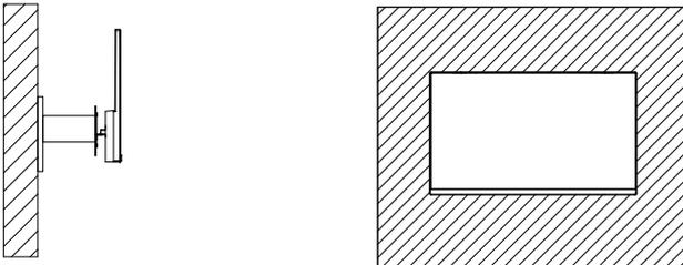
**⚠** Notes: To prevent the monitor on the mount from failing, please install it firmly and protect it fully. Do not place or hang any object on the mount, and the using height of the mount should be less than 2 meters.
