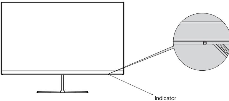
6. Indicator: Steady blue light indicates the power is on and the monitor runs normally. Red light indicates no video source and no horizontal or vertical signal detected or low voltage. Please make sure that your computer is turned on and all video cables are fully plugged in and/or connected.
