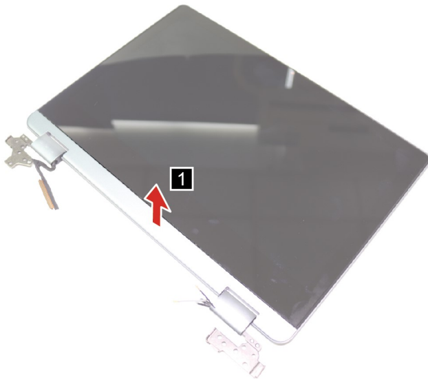
Figure 21. Remove the strip cover
