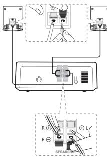
2. Connect the wireless receiver and the rear speakers (left, right) with the speaker cables.
