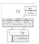
When you mount it on a wall (concrete), use the wall plugs. You should drill some holes. A guide sheet (Wall bracket install guide) is supplied to drill. Use the sheet to check the point to drill.
