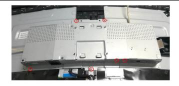
Take off the tapes and remove the Mylar. Disconnect the pin. Take off the tape and remove All screws. Tool : Screwdriver #2 Disconnect all the pins
