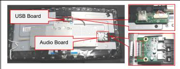
Remove the screw\*6 pcs to remove the mainframe.
