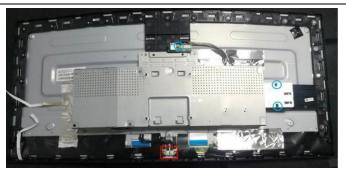
Disconnect the connectors to remove the USB board and the Audio board.
