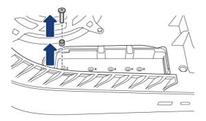
Move the spacer to the groove marked "80".
