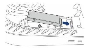
Important Make sure Game Drive PS5 NVMe SSD is inserted all the way into the expansion connector before proceeding to the next step. If Game Drive PS5 NVMe SSD is incorrectly inserted, it may cause damage to the terminal and your console.
