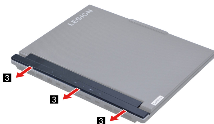
Figure 52. Remove the strip cover
