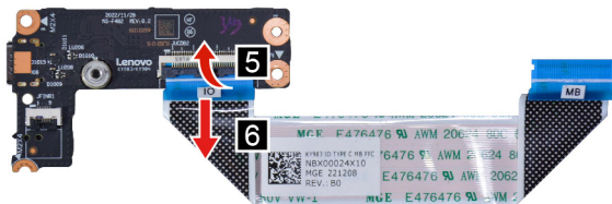
Figure 25. Remove the Type-C board cable
