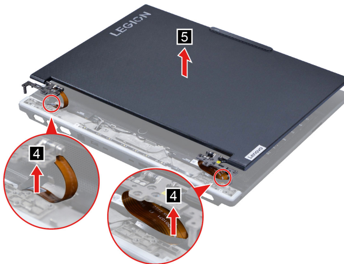
Figure 55. Remove the LCD module
