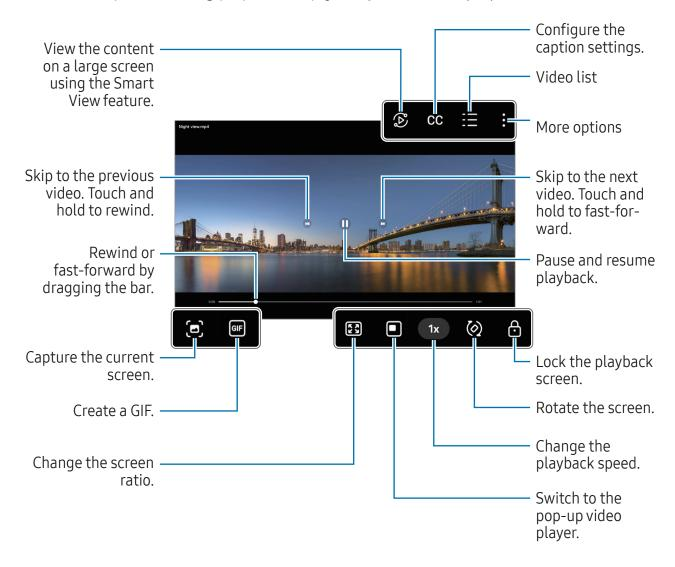
Drag up or down on the left side of the playback screen to adjust the brightness, or drag up or down on the right side of the playback screen to adjust the volume.
