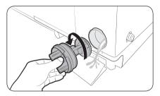
1. Put a floor-cloth or towel under the Pump filter. Turn the filter knob anticlockwise to remove.
