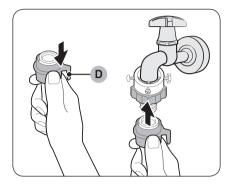
While pulling down part (D) on the water hose, connect the water hose to the adaptor. Then, release part (D). The hose fits into the adaptor with a clicking sound.
