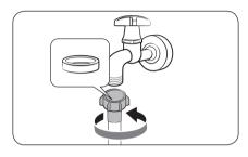
1. Connect the water hose to the water tap, and then turn the connector clockwise as shown.
