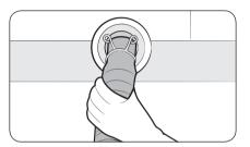
2. Insert the drain hose into the drain outlet. Make sure to connect them firmly using the joint ring. The drain hose is extensible. Adjust the length of the drain hose as needed.
