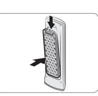
When cleaning is complete, close the cover and reinsert the filter case to the original position. You will hear a clicking sound when the filter case fits in.
