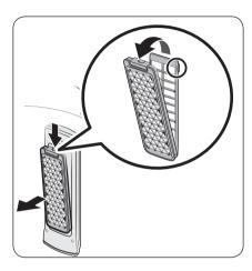
1. Press down the upper area of the filter case to remove.
