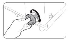
**3.** Reinsert the filter, and turn clockwise until it locks into position.
