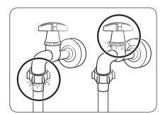
**3.** Open the water tap and check if there are any leaks around the connection areas. If there are water leaks, repeat the steps above.
