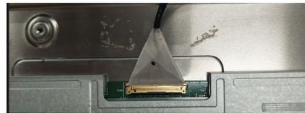
**S14** Unlock 7 screws to disassemble Middle Frame and “ASSY BKT CHIN” (See blue marks)
