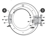
5 Remove the door catch **6** from the appliance frame by removing 2 screws and then assemble them on the opposite side.
