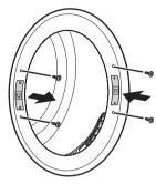
7 Install the door with the screws removed in step 1 and then check the door closes properly.
