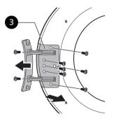
3 Remove the 3 screws from the door latch assembly **4** which is fixed between the door
