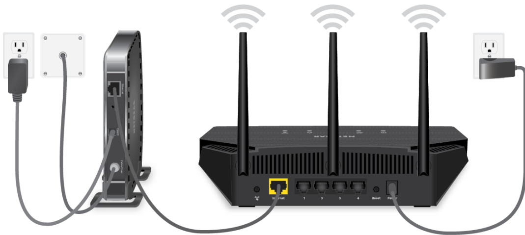
Figure 6. Cable your router
