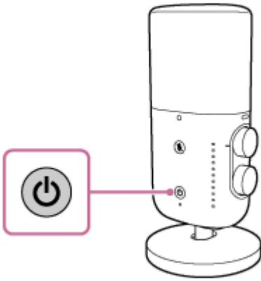
Immediately after the receiver and the microphone are turned on, the LINK lamp on the microphone starts blinking slowly in blue. This indicates that each of the devices is making a series of attempts to detect, connect to, and authenticate the other device. When a connection is established between the devices and clear audio recording is possible, the LINK lamps on both devices stay lit in blue.
