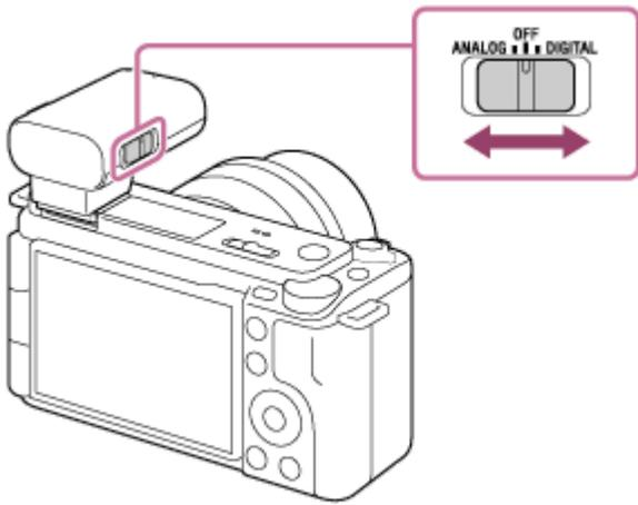
If your camera is compatible with the digital audio interface of the Multi Interface Shoe, make sure that the switch is set to “DIGITAL.” If not, set the switch to “ANALOG.”
