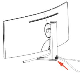
8. Cables can be connected through decorative holes in the bracket.
