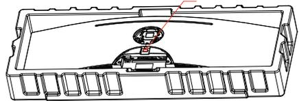
6. When detaching the base, remove the semicircular cover first, then press down the quick release button as illustrated.
