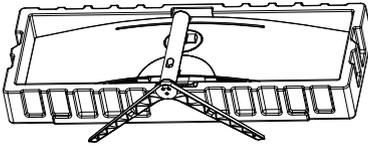
5. Attach the base of step 4 to the quick release notch of the LCD monitor securely.
