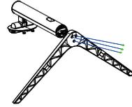
4. Tighten the base and stand arm with three screws.
