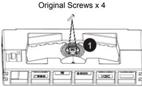
1. Remove the original screws x 4 Fig. 1 from the opening back of the monitor.
