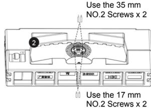
2. Tighten the two types of NO.2 screws as Fig. 2.
