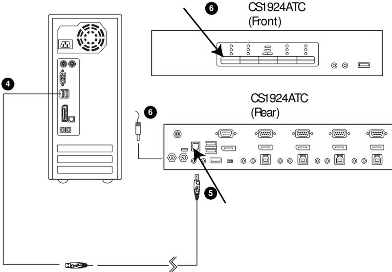
5. Connect the other end of a self-supplied USB Micro-B cable to the unit's USB Micro-B port.
