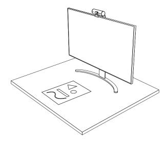
2. If mount is not secured with micro-suction pad: Hold the mount still with one hand and tilt the camera up or down with the other.
