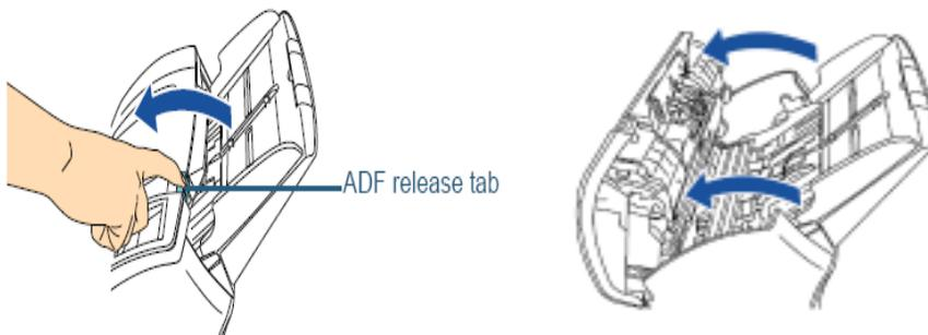
Open the sheet guide by lifting the tab
