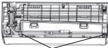
Orifices de drainage
