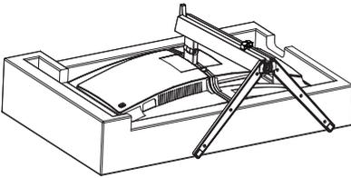
2. While keeping the release button pressed, tilt the stand and slide it out.
