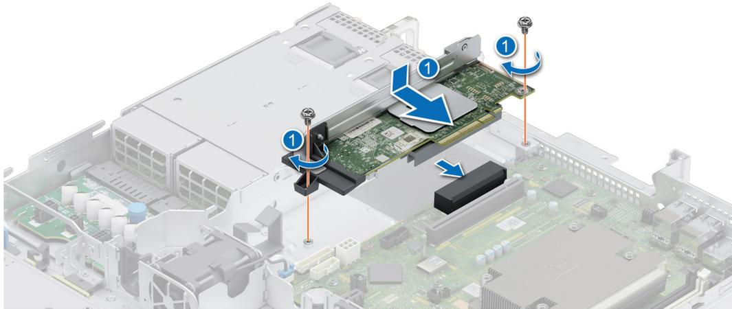
Figure 64. Installing the PERC card
