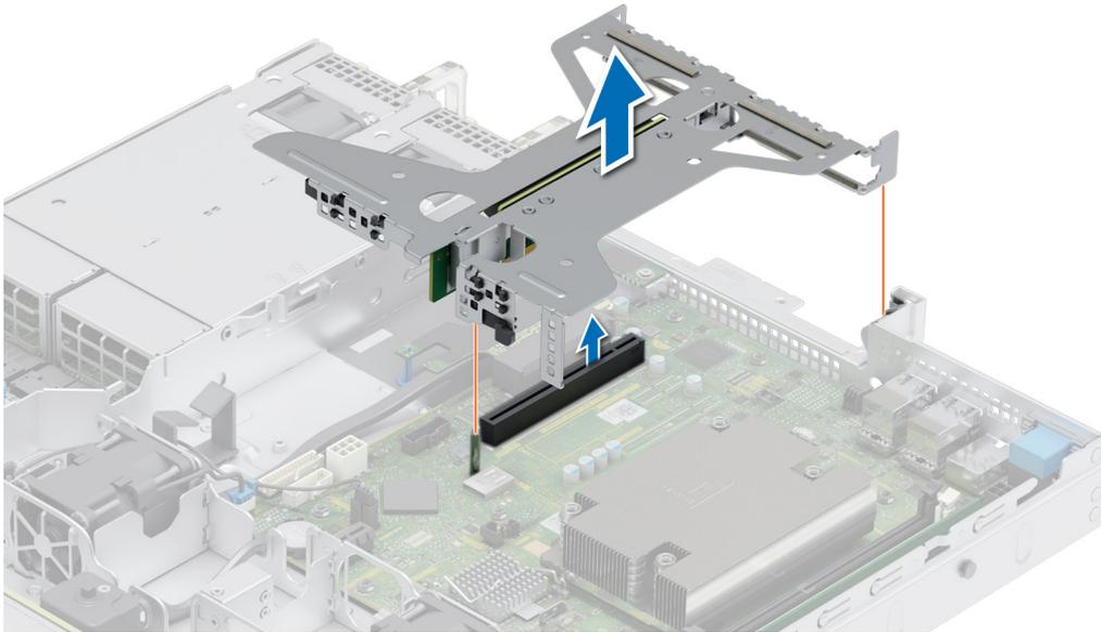
**Figure 47. Removing the butterfly riser**
