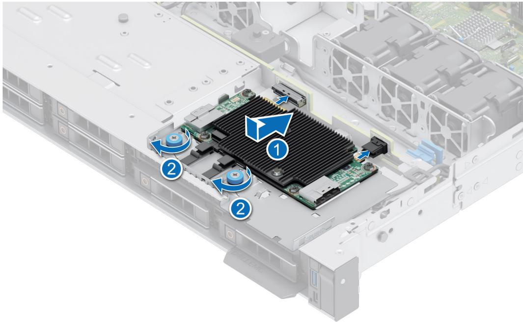
**Figure 62. Installing the front mounting front PERC module**
