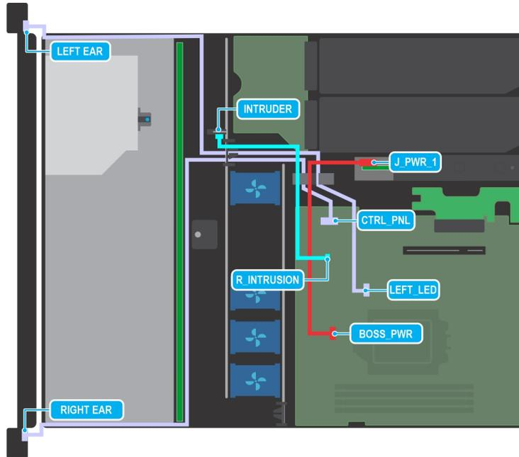
**Figure 24. Cable routing - 4 x 3.5-inch drive SAS or SATA backplane with butterfly riser, BOSS card**
