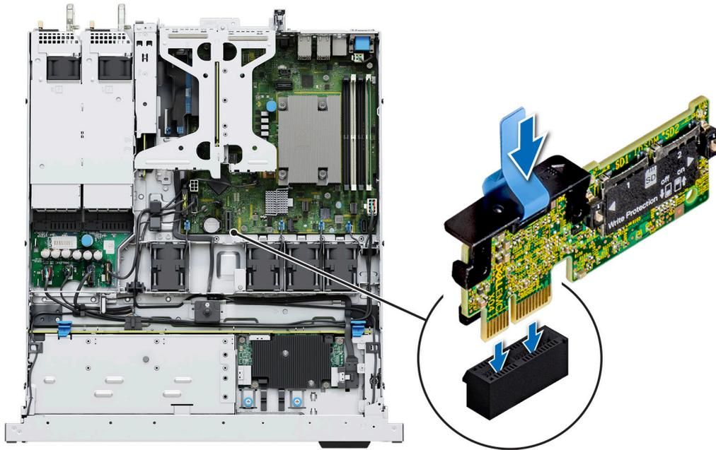
Figure 74. Installing the IDSDM module
