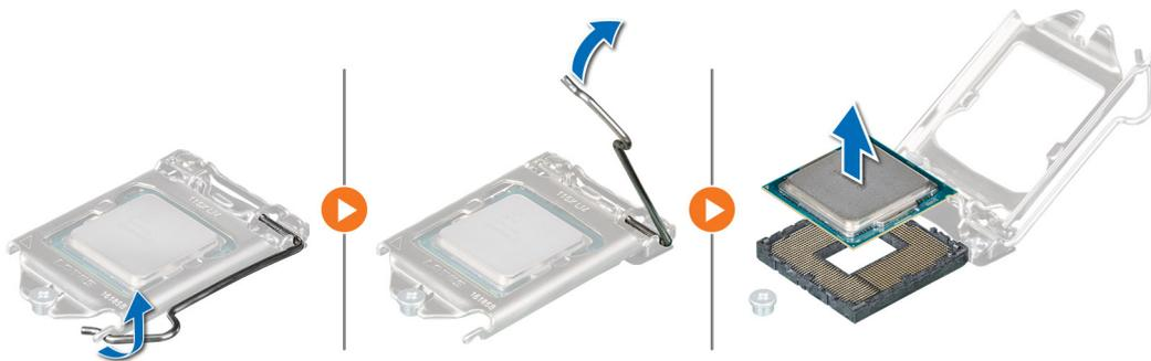
Figure 43. Removing the processor
