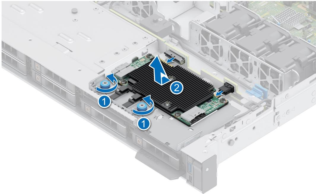
**Figure 61. Removing the front mounting front PERC module**
