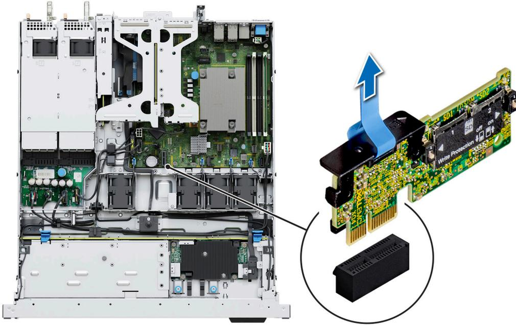
**Figure 73. Removing the IDSDM module**
