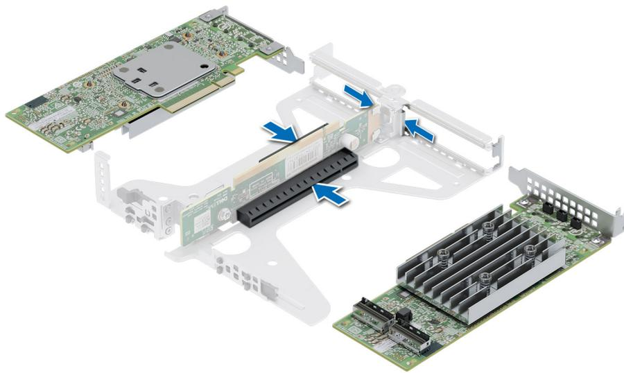
**Figure 52. Installing an expansion card into a riser**
