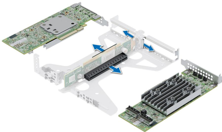
**Figure 49. Removing an expansion card from riser**
