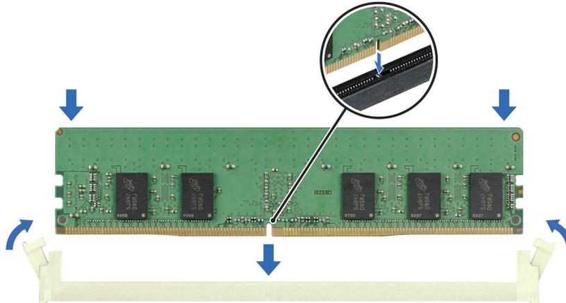
**Figure 39. Installing a memory module**
