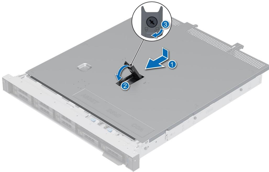
**Figure 12. Installing the system cover**
