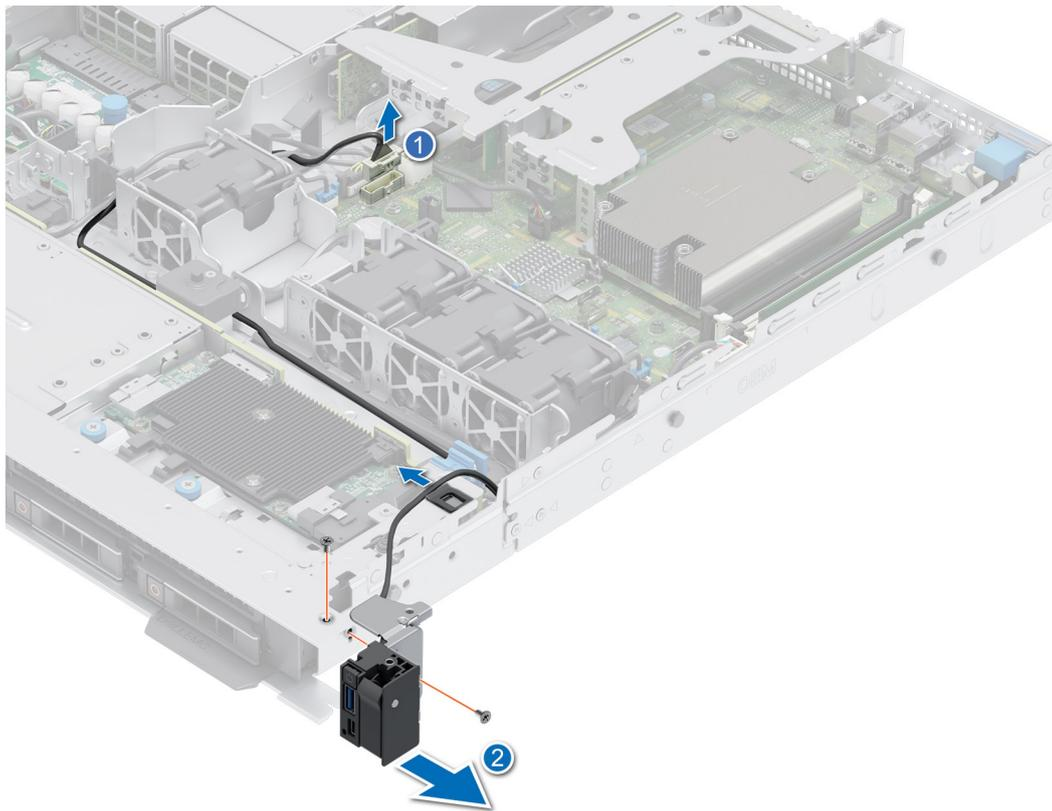
**Figure 82. Removing the right control panel**
