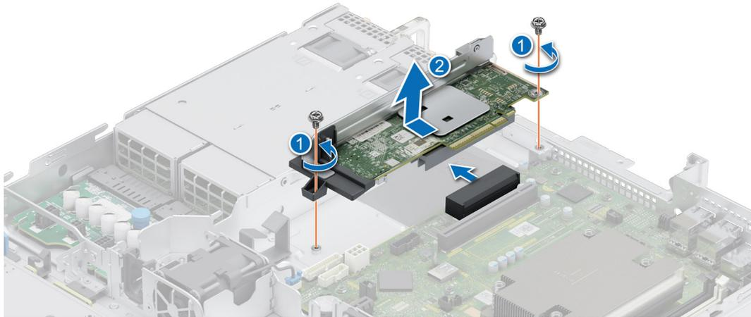
**Figure 63. Removing the PERC card**
