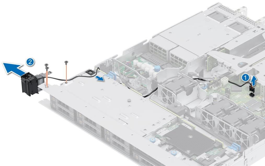
**Figure 80. Removing the left control panel**
