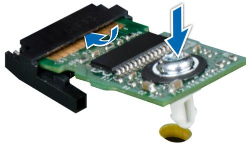
Figure 79. Installing the TPM
