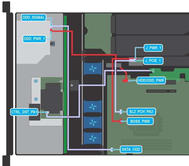
Figure 25. Cable routing - 4 x 3.5-inch drive SAS or SATA backplane with fPERC, and BOSS card
