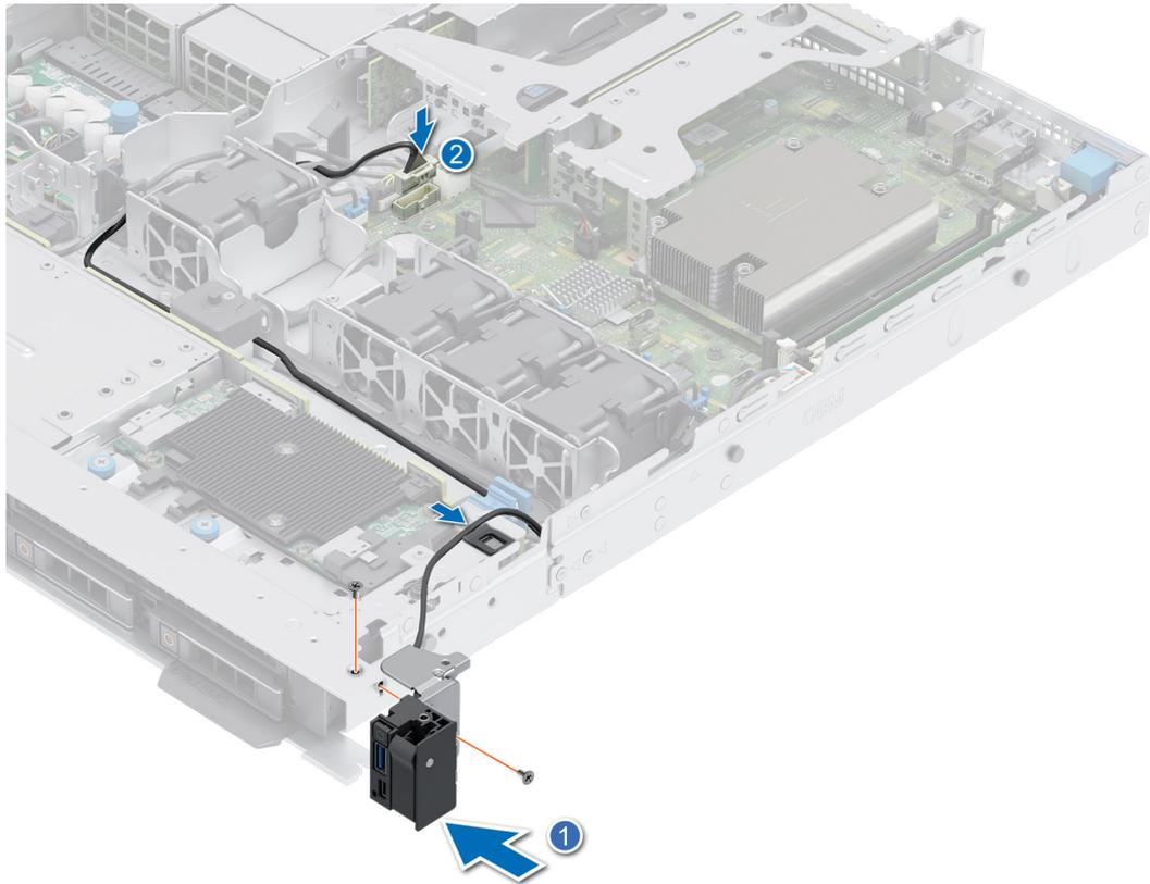
**Figure 83. Installing the right control panel**
