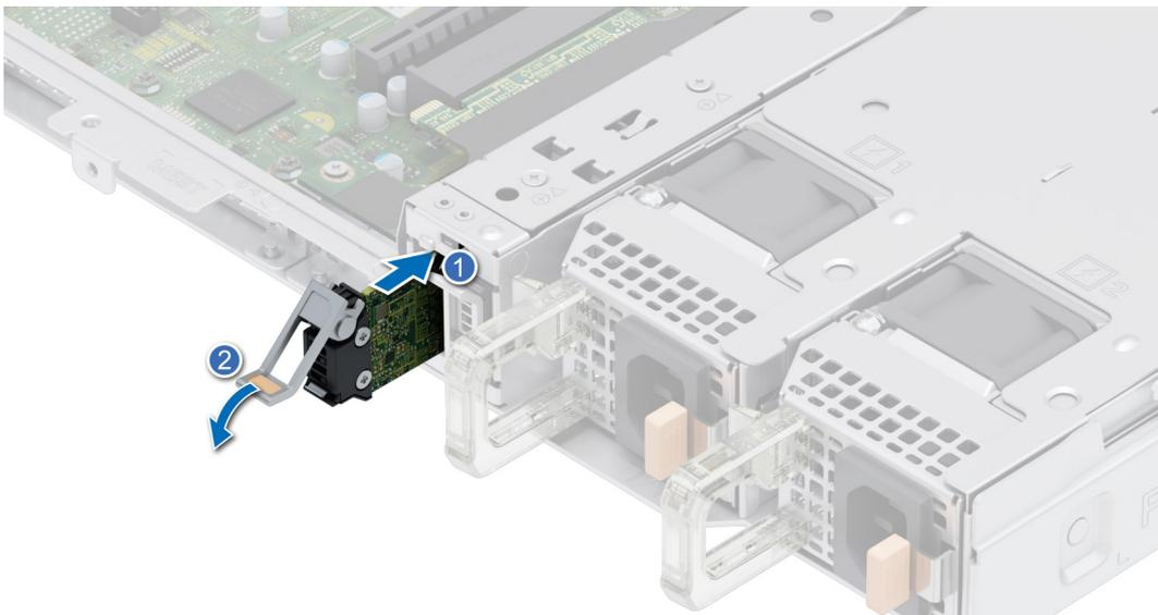
**Figure 58. Installing the BOSS S2 card carrier**
