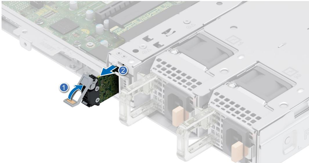
**Figure 53. Removing the BOSS S2 card carrier**
