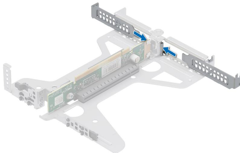
**Figure 50. Installing filler bracket in the riser**
