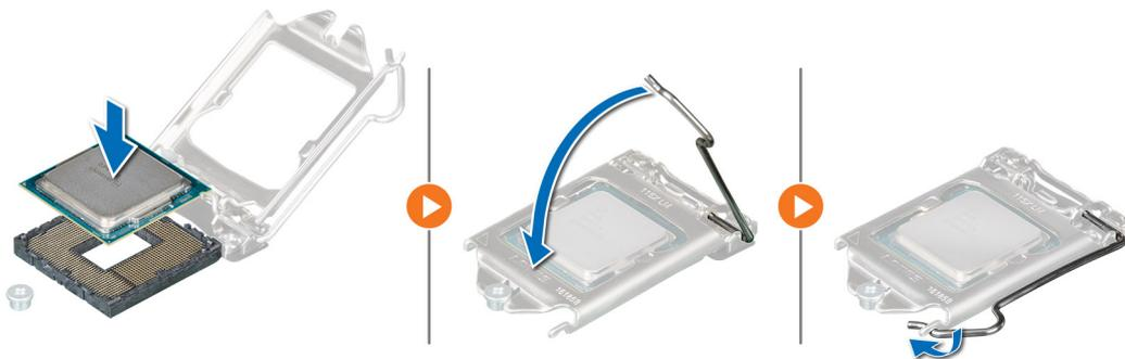
Figure 44. Installing the processor
