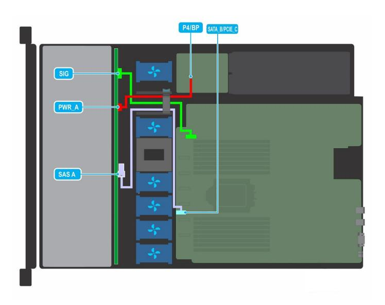
Figure 1. Cable routing -  $4 \times 3.5$  inch SATA drive backplane
