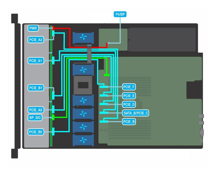
Figure 2. Cable routing - 10 x 2.5 inch NVMe drive backplane
