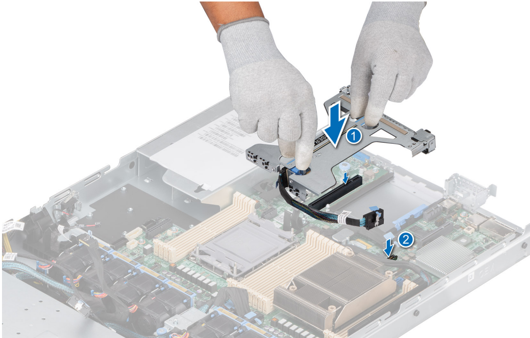
Figure 75. Installing the Riser 2b with SNAP! module
