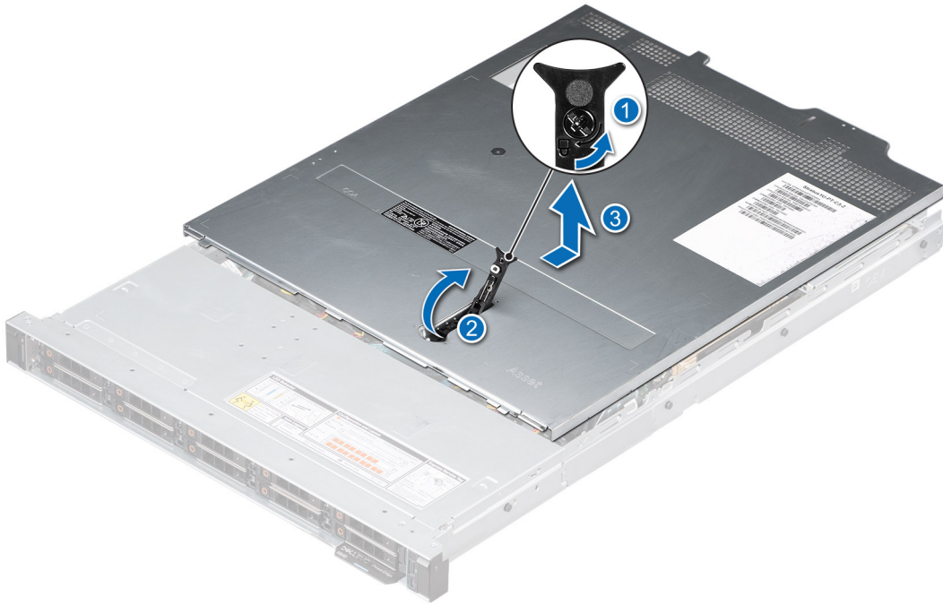
Figure 14. Removing the system cover
