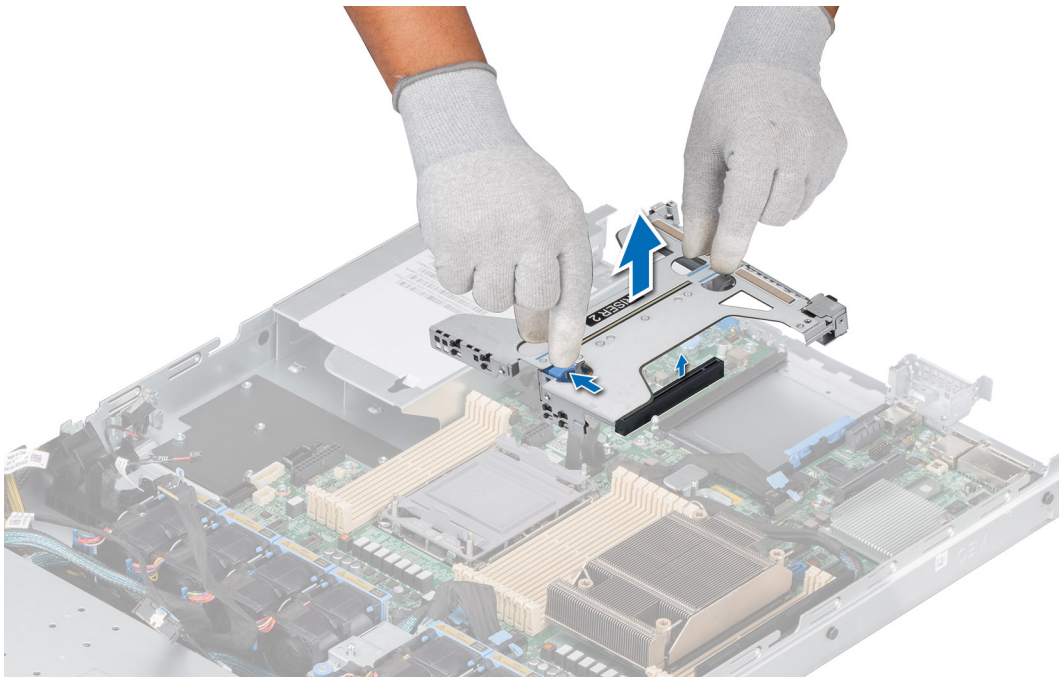
Figure 72. Removing the Riser 2c
