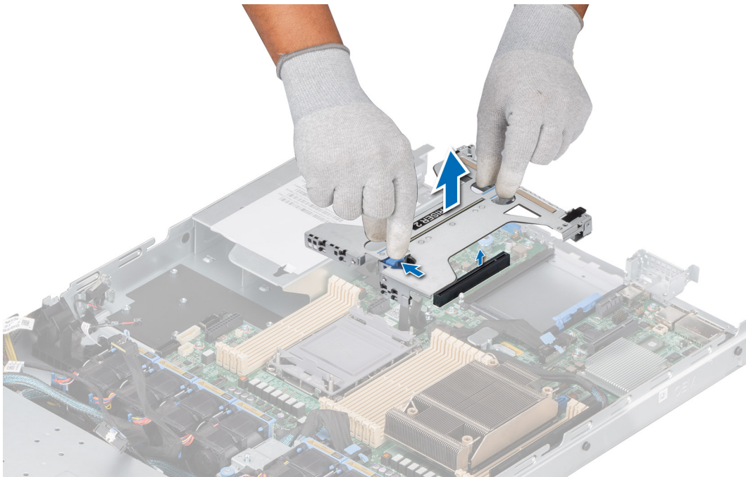
Figure 70. Removing the Riser 2a
