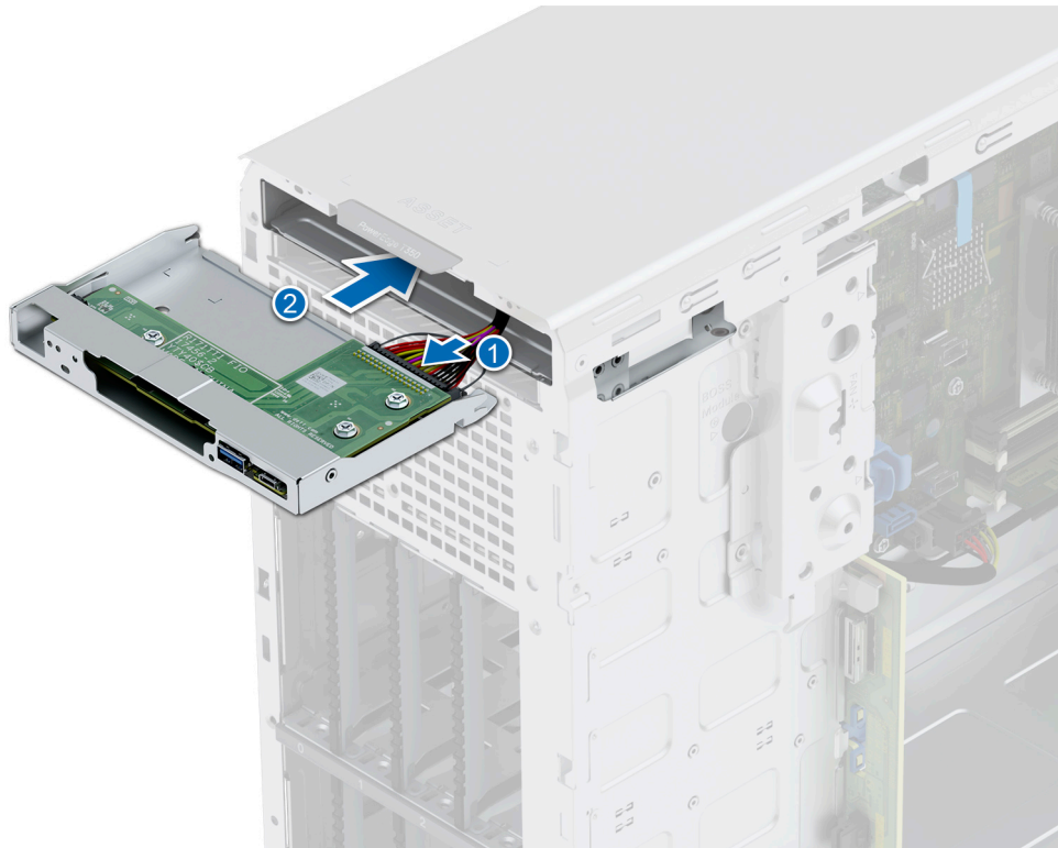
Figure 99. Installing the control panel cage
