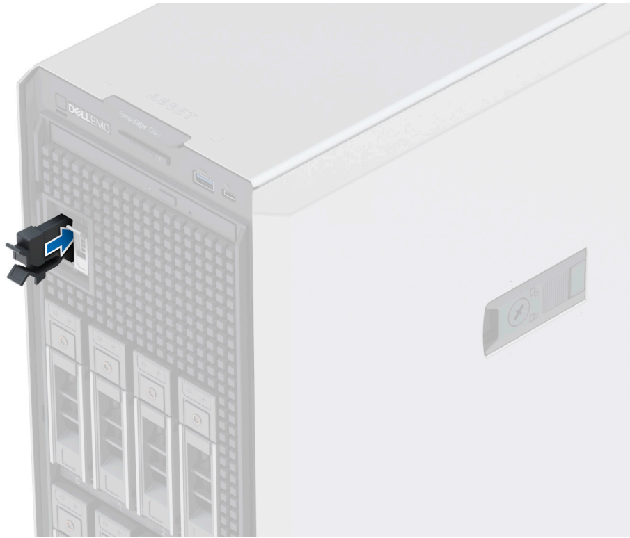
Figure 62. Installing the BOSS S2 card carrier blank
