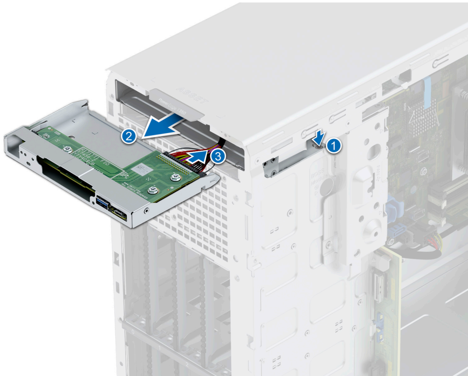
Figure 96. Removing the control panel cage
