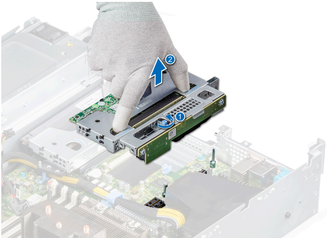
Figure 67. Removing the riser 1A
