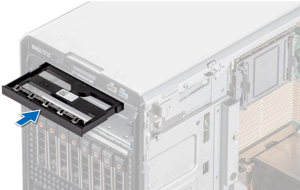
Figure 96. Installing the optical drive blank
