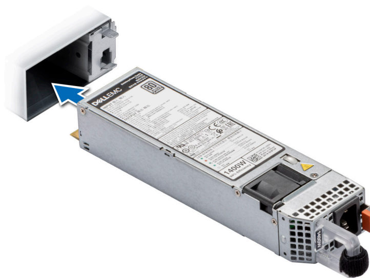
Figure 173. Installing a 60 mm power supply unit
