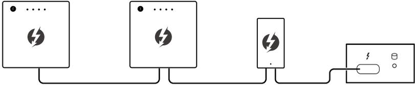
You can also daisy-chain monitors on the front IO panel. Please note that monitors should be the last devices on the chain.
