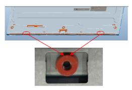
S19 Disassemble mylar from Main SHD
