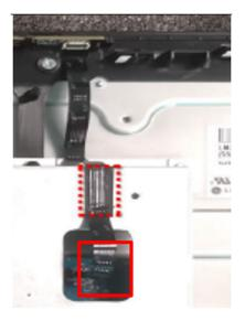
S8 Disassemble "SENSOR BD" from Middle Frame
