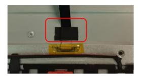
**S16** Unlock 11 screws to disassemble Middle Frame (See red mark)
