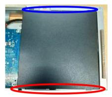
S20 Unlock 10 PCBA screws to disassemble I/F BD, SPS BD and LED Driver BD from Main SHD
