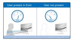
PowerSensor is a built-in 'people sensor' that transmits and receives harmless infrared signals to determine if the user is present and then automatically reduces monitor brightness when then user steps away from the desk, cutting energy costs by up to 80 percent and prolonging monitor life
