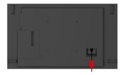
Use a screwdriver to remove 16pcs screws for releasing the handles. (Torque:15±0.5kgf) Remove 6pcs screws for unlocking IO hing with rear cover. (Torque:3±0.3kgf) Remove 69pcs screws for unlocking the rear cover(Torque: 3±0.3kgf).
