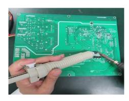
S25-5 Lift the bulk cap. up and away from the PCB.
